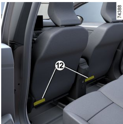
Footwell heater outlets for occupants 12 .
