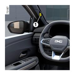
The system analyses the behaviour of the driver's face using the interior camera 1 and emits a warning if there is a risk of the driver falling asleep.
