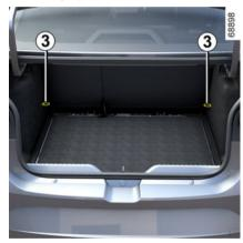
The anchorage points 3 located in the luggage compartment allow loads to be secured.
