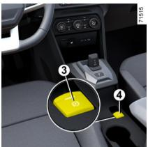
You can apply the electronic parking brake manually.
