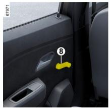
Turn the handle **8** to lower or raise the window to the desired height.
