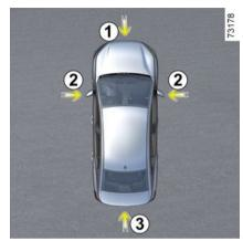
If fitted on the vehicle, the four cameras 1, 2 and 3 located in the front bumper, door mirrors and tailgate help you with difficult manoeuvres.
