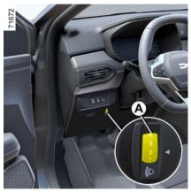
Control **A** is used to adjust the height of the headlight beams according to the load.
