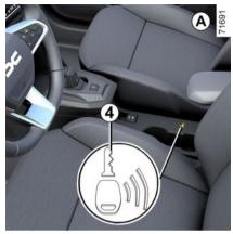
Press the brake or clutch pedal, then place the card 3 (A or B) on the symbol 4 (A or B). Press the button 2 to start the vehicle. The message goes out.
