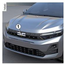
If the front camera is activated automatically or manually, the view from the camera is displayed on the screen 4.
