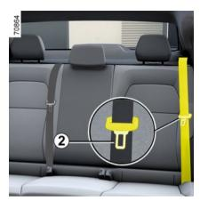
When installing for the first time, use the seat belt buckle 2 to cut the fusible seams of the slots marked by the sym-
