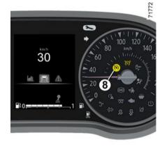
Depending on the vehicle, the warning light 8 disappears to confirm standby.
