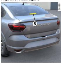
The bulb **9** of the high level brake light **8** can be accessed through the luggage compartment.
