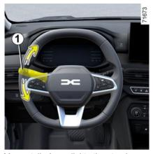
Move stalk 1 parallel to the steering wheel and in the direction you are going to turn it.
