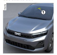
Using the information from the camera 1. this function informs the driver of the time interval between their vehicle and the vehicle in front so that a safe stopping distance between the two vehicles can be maintained.
