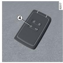
Press button 4 to switch on the interior lighting, the side lights and the dipped beam headlights for approximately 20 seconds. This can be used, for example, to identify your vehicle from a distance when parked in a car park.
