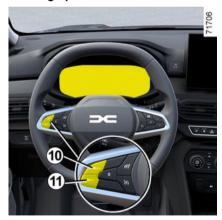
To adapt the speed limiter or cruise control setpoint to the detected speed
