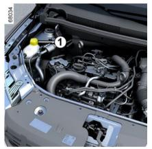
With the engine off and the vehicle on flat ground, the level when cold must be between the "MINI" and "MAXI" marks on the coolant reservoir
