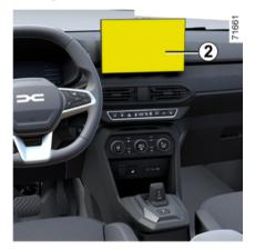
Vehicle stationary, engine on, from the multimedia screen 2, you can add or remove the guides and adjust the camera image settings (brightness, contrast etc.). Please refer to the multimedia instructions for further information.
