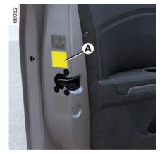
Open the driver's door to read it. Tyre pressures should be checked when the tyres are cold.
