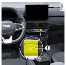
Press the switch 1 to deactivate the function. The "Stop & Start deactivated" message appears on the instrument panel and the switch 1 indicator light is lit.
