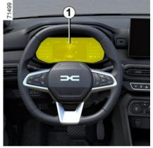
The system displays the current pressures on the instrument panel 1 and alerts the driver in the event of insufficient pressure.
