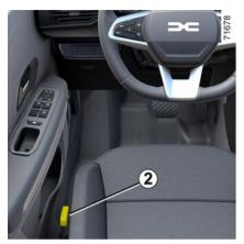
Depending on the vehicle, lift lever  $\boldsymbol{2}$  to unlock the fuel filler flap  $\boldsymbol{A}$ . Open it, then unscrew the fuel tank cap  $\boldsymbol{1}$ .
