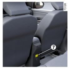
Multimedia sockets USB-C 2 and 7 (depending on the vehicle) can be used to charge accessories with a maximum power of 12 Watts (5 Volts) per socket.
