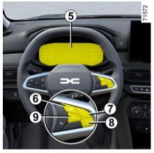
With the vehicle stopped, press the switch 6 as many times as re-
