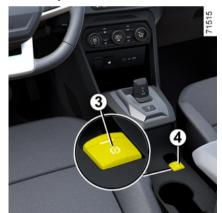
To apply the electronic parking brake manually (when stopping at a red light, stopping when the engine is running.
