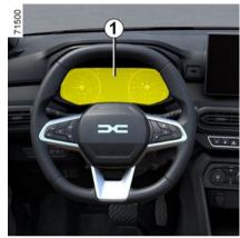
The information on the instrument panel signals any potential tyre pressure faults (e.g. deflated or punctured tyre). For your own safety.
