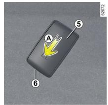
Slide the rear casing **5** downwards while pressing on area **A**.
