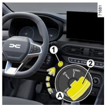
Applying the electronic parking brake
