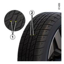
The tyres must be in good condition and the treads must have sufficient depth: tyres approved by our Technical Department have wear warning strips 1 which are indicators moulded into the tread at several points.
