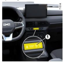
The indicator light 1 lights up when the ignition is switched on and goes out after a few seconds.
