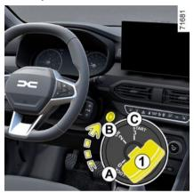
If the engine fails to start at the first attempt, turn the key back before activating the starter again.
