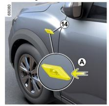
Unclip the direction indicator light **14** using a flat-blade screwdriver or simil-
