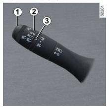
If fitted on the vehicle, the daytime running lights and rear side lights come on automatically without any action on the stalk 1 when the engine is started, and they go off once the engine is switched off.
