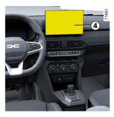
The cameras transmit four separate views to the screen 4, making it possible to view the area around the vehicle.
