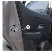
To make it impossible for the rear doors to be opened from the inside, move lever *3* on each door and check from the inside that the doors are securely locked.
