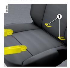
The two rings 1 are located between the seatback and the seat base and
