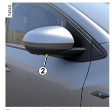
The cameras **2** installed in the door mirrors transmit the side views to the screen **4**.
