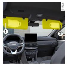
Lower the sun visor **1** or **2** over the windscreen or unclip it and flip it to cover the side window.
