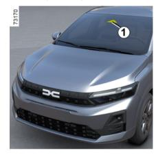
Using information from the 1 camera, the function triggers corrective action on the vehicle steering system when a continuous or broken line is crossed or when approaching the roadside (divider, barrier, pavement, embankment, etc.) without activating the direction indicator lights.
