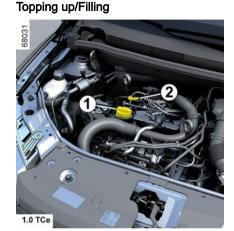
The vehicle must be parked on level ground and the engine should be stopped and cold (e.g. before the engine is started up for the first time that day).
