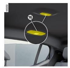
Using a flat-blade screwdriver or similar, unclip the rear courtesy light *16* by pressing the tab located on one side of the courtesy light to access the bulb.
