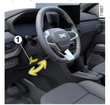
The steering wheel height and, depending on the vehicle, depth can be adjusted.
