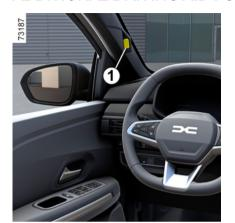
The system analyses the behaviour of the driver's face using the interior camera 1 and emits a warning if any distraction is detected.
