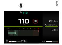
The green **7** warning light or, depending on the vehicle, the **6** or **8** warning light disappears from the instrument panel to confirm that the function is deactivated.
