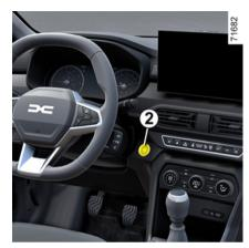
on vehicles with a manual gearbox, press the brake pedal or clutch and press button 2. If a gear is engaged, the vehicle may only be started by depressing the clutch pedal.
