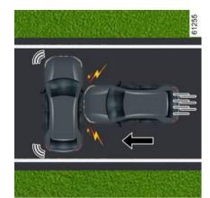
In a side impact with another vehicle of an equivalent or higher category, at an impact speed equal to or greater than 31 mph (50 km/h).
