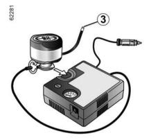
Once the tyre is correctly inflated, remove the kit: unscrew the inflation adapter slowly from the container 3 to prevent any product spatter and store the container in plastic packaging to prevent product leaks.
