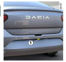
When reverse gear is engaged, the camera 1 located at the rear of the vehicle transmits a view of the area behind the vehicle to the multimedia display 2 accompanied by three guide lines 3, 4 or 5 (fixed, moving and trailer guide lines).
