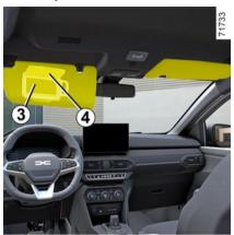
Depending on the vehicle, the sun visors are fitted with a courtesy mirror.
