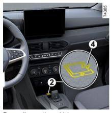
Depending on the vehicle, you can use the induction charging zone **2** to charge a smartphone without using a cable.
