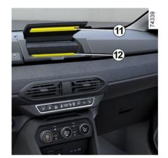
Make sure that the telephone is securely held in place between the 11 and 12 stands before use.
