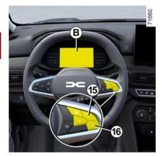
Depending on the vehicle, use control **15** or **16** to browse and select the various widgets on the instrument panel:
