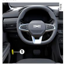
To open the bonnet, pull the handle 1 located on the left-hand side of the dashboard with a door open.
