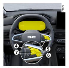
With the vehicle stationary, press the switch 4 as many times as re-
