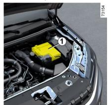
The battery 1 does not require maintenance. You should not open it or add any fluid.
