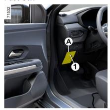
If any electrical component does not work, check the condition of the fuses. Unclip the flap **A** using the notch **1** or, depending on the vehicle, unclip the flap **B** using the notch **2**.
