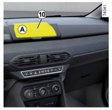
On vehicles that are equipped, lift the flap 10, place your phone 13 horizontally onto the stand 11 then lower the flap 10 while keeping the phone in position on the stand 12.
