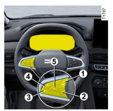
The speed limiter function helps you stay within the driving speed limit that you choose, known as the **limit** speed.
