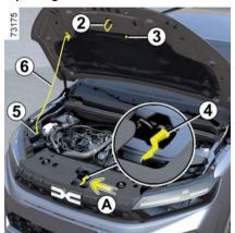
Raise the bonnet and disengage the stay 6 from its mounting 3; for your own safety, place the stay in its retainer 5.
