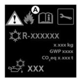
The refrigerant fluid circuit (of which some components are hermetically sealed) may contain fluorinated greenhouse gases.
