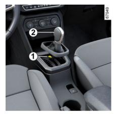
When setting off, if the lever is locked in position **P** when you press the brake pedal (e.g. battery fault), it is possible to manually release the lever to unblock the drive wheels. To do this, unclip the base of the gaiter and press the 1 push button while simultaneously pressing the 2 button on the lever to unlock the lever and shift to position **N**.
