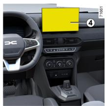
Automatic mode is activated when reverse gear is engaged and the screen 4 shows the rear camera view. When there is a quick change from reverse gear to forward gear, the screen 4 shows the image transmitted from the front camera.
