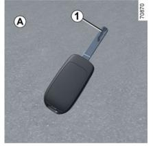
1. Coded key for starter ignition switch, doors, fuel filler cap and, depending on the vehicle, the luggage compartment only.
