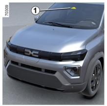
Using information from the 1 camera, the function triggers corrective action on the vehicle steering system when a continuous or dashed line is crossed or when approaching the roadside (divider, barrier, pavement, embankment, etc.) without activating the direction indicator lights.
