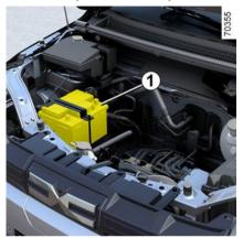
The secondary battery is a 12V battery: this supplies the energy reguired to operate vehicle equipment (lights, windscreen wipers, audio system, etc) and certain safety systems, such as ABS
