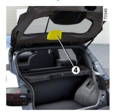
The bulb for high-level brake light **4** may be accessed through the boot. Slide the bulb cover downwards to release it.
