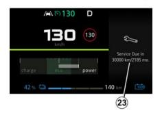
Remaining distance for maintenance and Remaining days for maintenance 23
