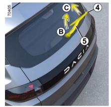
With the wiper in the park position and the ignition off, lift wiper arm 5. Pivot wiper blade 4 until some resistance is met (movement B). Pull the blade (movement CB). Pull the blade (movement C) to release it.
