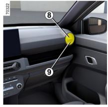
To open, press the ventilation outlet **8** until it opens as far as required.
