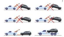
Breakdown recovery **must** be performed on a flat surface under all circumstances except where the vehicle is immobilised following a full discharge of the traction battery. In the event of a total energy loss, please see the following pages.
