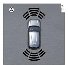
Most obstacles located near the rear and, depending on the equipment, the front of the vehicle are detected.
