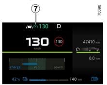
Press switch 3 as many times as necessary until the light 7 lights up grey on the instrument panel.
