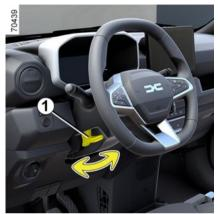
Depending on the vehicle, the steering wheel height are adjustable.
