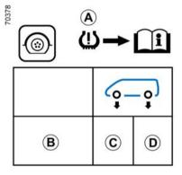
B. : dimension of the tyres fitted to the vehicle.
