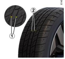
The tyres must be in good condition and the tread form must have sufficient depth; tyres approved by our Technical Department have tread wear indicators 1 which are indicators moulded into the tread at several points.
