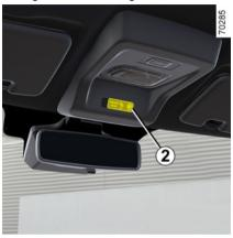
To deactivate the airbag: stationary vehicle ignition switched off, push and turn lock 1 to the OFF position. With the ignition on, you must check
