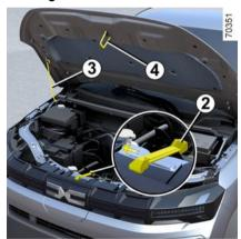
To close the bonnet, remove the Stay rod *3* from the hole and place to the lock clip. Lower it to 30 cm above the closed position, then release it. It will
