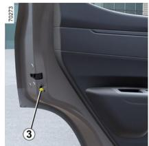
The child safety lock prevents the rear doors from being opened from the inside. Move lever 3 on each rear door
