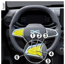
While the vehicle is moving a steady speed (above approximately 19 mph (30 km/h)), press the switch *6* (SET/-) or the switch *1* (SET/+): the function is activated and the current speed is taken into account.
