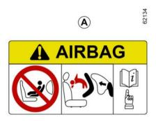
The markings on the dashboard and labels **A** on each side of the passenger sun visor **3** (example : label shown above) remind you of these instructions.
