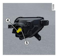
Remove bulb connector 4.Unclip spring 5 and take out the bulb.
