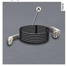
This cord is specific to your vehicle and designed for connecting to wall sockets or public terminals to enable standard charging of the traction battery.
