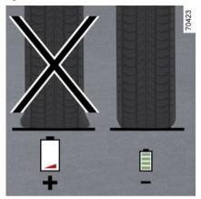
An under-inflated tyre increases energy consumption. Comply with the specified tyre pressures for your vehicle.
