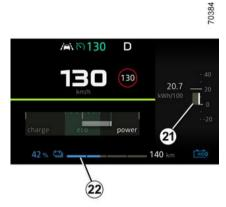
Consumption widget page displays the Instant consumption gauge 21 SOC (State of charge) bar displays the Current level of vehicle battery available charge 22
