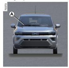
The QR Code on the label **A** allows emergency workers using a tablet or smartphone to immediately access the technical information useful for working on the vehicle in the event of an accident
