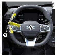
Press the steering wheel boss **A** to activate the horn.
