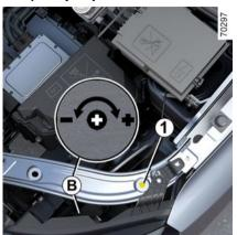
Open the bonnet and identify the marking **B** next to one of the front headlight projectors.
