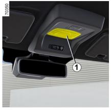
Release the courtesy light 1 with a tool such as a flat-blade screwdriver.
