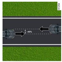
In a frontal impact with another vehicle of an equivalent or higher category, with an impact area equal to or greater than 40 %, where the speed of both vehicles is equal or greater than 25 mph (40 km/h).
