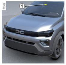
The system displays speed limits on the instrument panel according to road signs detected on the side of the road.
