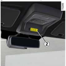
To reactivate the airbag: vehicle stationary, ignition switched off, press and turn the lock to 1 position ON.
