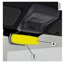
The interior rear-view mirror 4 is manually adjustable. When driving at night, tilt the mirror by lever 5 or by hand to avoid being dazzled by the headlights of the vehicle behind.
