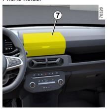
On vehicles that are equipped, lift the flap **7**, place your phone **10** horizontally onto the stand **8** then lower the flap **7** while keeping the phone in position on the stand **9**.
