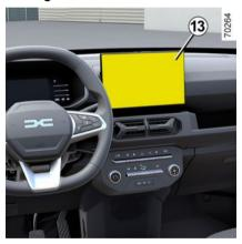
You can set the threshold's value for the minimum traction battery charge level from the multimedia screen 13 For more information, refer to the multimedia manual.
