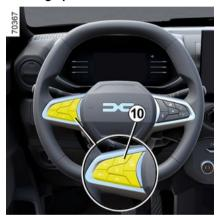
To adapt the speed limiter and cruise control setpoint to the detected speed limit, press the 10 switch.
