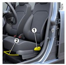
Lift knob 1 upward to unlock recliner mechanism. Tilt the seat back to desired position and release knob. Ensure seat back is locked properly after release.
