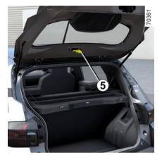
Turn the bulb holder **5** a quarter of a turn, release it and remove the bulb.
