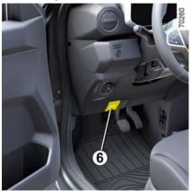
pull the button 6 to unlock the charging flap 9;
