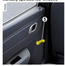
Turn the handle **5** to lower or raise the window to the desired height.
