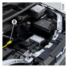
The « 260 V » electrical circuit is denoted by orange cables **8** and parts bearing the symbol.
