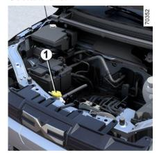
Check the level on flat ground, with the engine switched off. When cold, the level must be between the « MINI » and « MAXI » marks on the reservoir 1.
