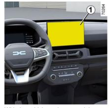
With the vehicle stationary and the engine on, select « Electric » from the « Vehicle » world on the multimedia screen 1, then select « Charging & Air conditioning » tab to access the settings.
