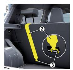
Pass the belt 2 between the seatback and the luggage compartment cover. To do so, first remove the luggage compartment cover. Attach the belt hook to one of the rings 3, indicated
