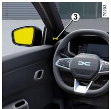
Adjust the door mirror according to rear vision by adjusting the knob 3
