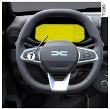
The following table lists the warning messages that appear on the instrument panel 7 when the system detects a tyre pressure fault.
