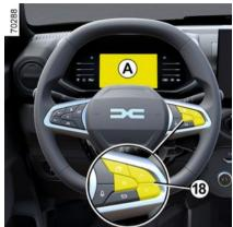
**Information area 17**, depending on the vehicle, browse using the control **18** to select various widgets on the instrument panel **A**:
