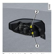
Turn bulb holder 2 or 3 and pull it out. Direction indicator light 2.Bulb type: WY16W.
