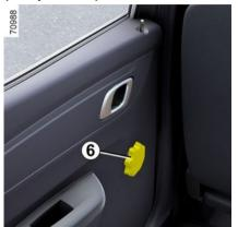
Depending on the vehicle, turn the rotary control *6* in anti-clockwise direction to lower or in clockwise direction to raise the window to desired height.
