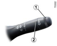
With the ignition on, turn the end of stalk 1 to align the symbol with mark 2.
