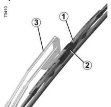
With the windscreen wipers in the off position and the ignition switched off, raise the windscreen wiper blade arm, 3, press the tab 2 and push the blade downwards to release it from its housing.
