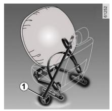
The pretensioners hold the seat belt against the body, holding the occupant more securely against the seat, thus increasing the seat belt's efficiency.
