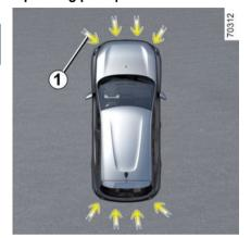
Ultrasonic sensors, indicated by arrows 1, are fitted in the bumpers to detect obstacles near the vehicle.
