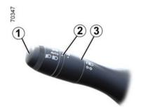
If fitted on the vehicle, the daytime running lights come on automatically with no action on stalk 1 when the engine is started, and they go off once the engine is switched off.
