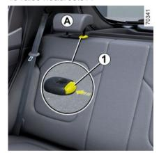
Pull the headrest upwards to the desired height.
