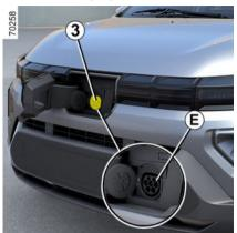
**Note:** If in a snowy environment, remove snow from the vehicle charging area before plugging in or disconnecting. Snow in the socket may block the insertion of the charging cord plug.
