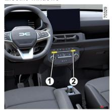
Press the bottom of switch 1 or 2 to open the window or press the top of switch 1 or 2 to close it to the desired level.
