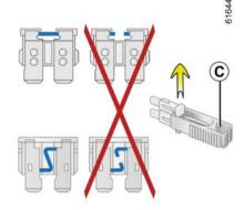
Remove the fuse using tweezers **C**located at the back of flap **A** or **B**.
