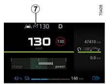
Press switch 3 as many times as necessary until the light 7 lights up grey on the instrument panel. The « Limiter ON» message appears on the instrument panel accompanied by dashes to indicate that the speed limiter function is activated and waiting for a limit speed to be stored.
