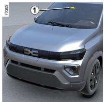
The system uses information from the camera 1, to determine the distance from your vehicle:
