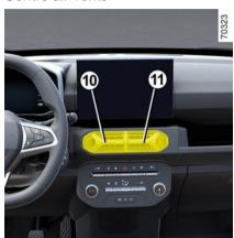
To adjust the airflow, move slide **10** or **11** up, down and sideways, until it opens as far as desired
