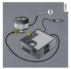
Once the tyre is correctly inflated, remove the kit: unscrew the inflation adapter slowly from the container 3 to prevent any product spatter and store the container in plastic packaging to prevent product leaks.
