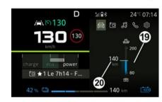
EV Autonomy widget page displays the bar of autonomy minimum and maximum range 19
