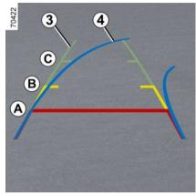
This is shown in blue on the multimedia screen 2. It indicates the vehicle trajectory according to the position of the steering wheel.
