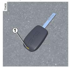
Open the case at slot 1 using a flat blade screwdriver or similar, and replace the battery 2, observing the type and polarity shown on the back of the cover.
