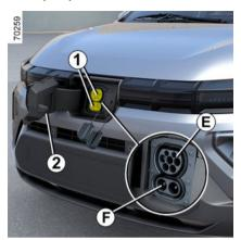
The vehicle is equipped with two charging connections located at the front of the vehicle:
