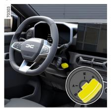
To lock: remove the key and turn the steering wheel until the steering column locks.
