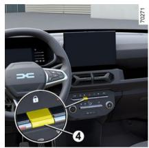
By pressing 4, It simultaneously locks or unlocks all the doors/tail gate and the charging gets stopped (when charging).
