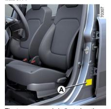
The tyre pressure is indicated on the label A affixed to the front driver. Tyre pressures should be checked when the tyres are cold.
